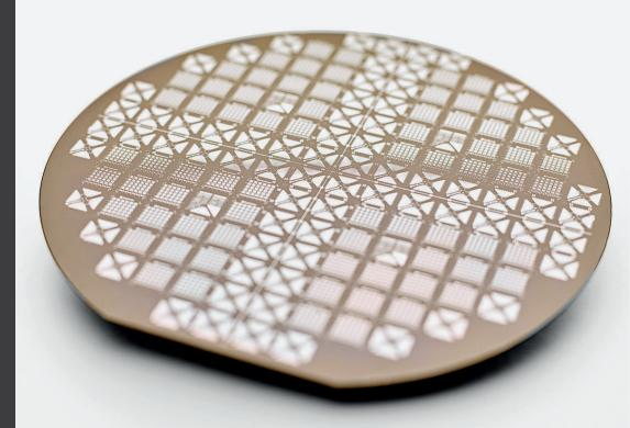
Graphenea offers Graphene Foundry Services on custom wafers up to 6" with customized design and materials. This enables fast device prototyping and accelerates the development towards your graphene-based application.
